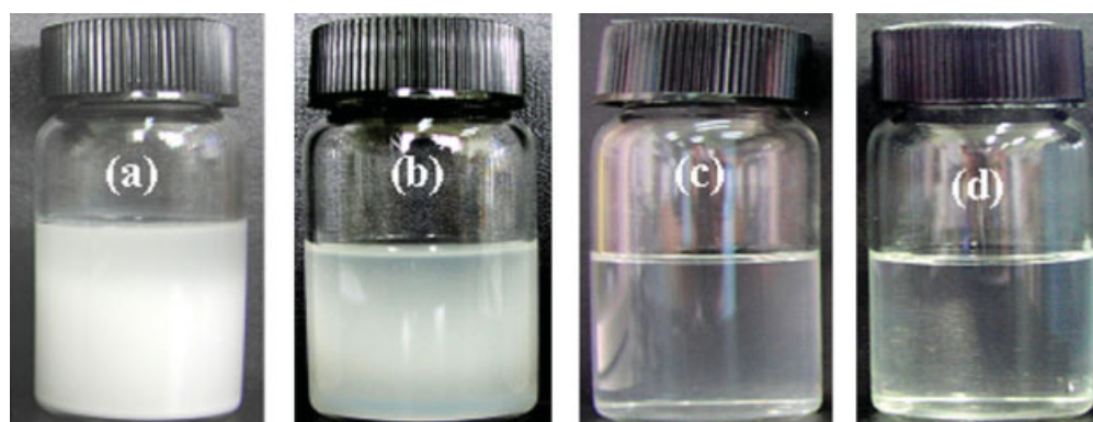
Figure 5 Digital photographs showing the state of the EVOH/SiO 2 hybrids gels with different IPTES contents: (a) 0, (b) 0.003, (c) 0.006, and (d) 0.012 mol. [Color figure can be viewed in the online issue, which is available at www.interscience.wiley.com .]
